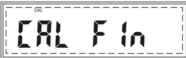
*Display indicating the calibration process is finished*
