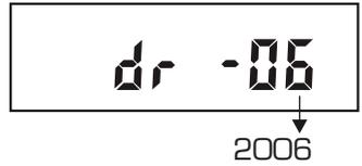
16. The scale will then begin to adjust the first digit of the year. Per our example, if the year setting is 2006, set the first digit at 0 by pressing the T key while 0 is displayed.
