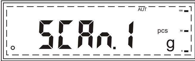
6. Scan the first NDC code by placing it slowly under the scanner light.
