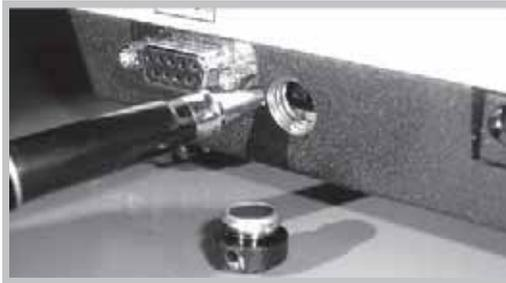
3. Upon toggling of the calibration switch, the balance will go into Calibration Mode. For approximately five (5) seconds the display will read CAL, indicating the scale is in Calibration Mode.
