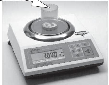
10. The weight of the sample will be displayed as it is placed on the pan.
