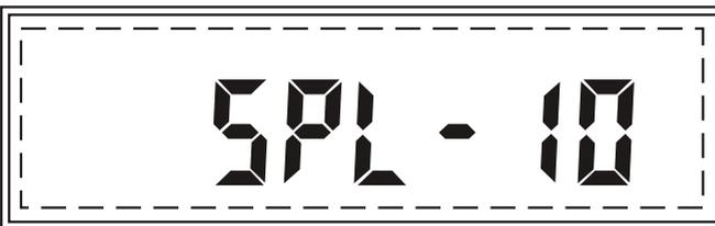
6. Once the new sample size has been selected, press the T button to confirm the new sample size selection. The display will now read SAPL On, indicating you should to place a new sample of 10 pieces on the pan (if SPL-10 is selected).
