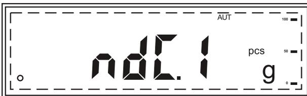
**Note:** Once NDC Verification has been enabled, anytime performing the counting operation two NDC codes must be scanned to allow the scale to check whether there is a match between the two codes.
