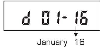
13. Now select the desired month. Press the T key while a number of the desired month is displayed. Per our example, press the T key while the number 2 for February is displayed.
