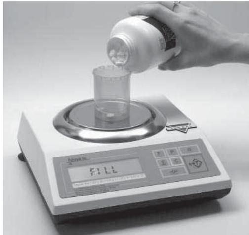
**Note:** If filling does not begin while the command "Fill" is displayed, after approximately 5 seconds the scale will display 10 pcs and will begin waiting for the count to begin.
