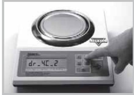
2. The scale will then display commands Set-t-0, and Set-t-1 appearing sequentially approximately every 2 seconds. To change the date and time, press the "T" key while command Set-t-1 is displayed. If you want to cancel the operation, press the T key while Set-t-0 is displayed.
