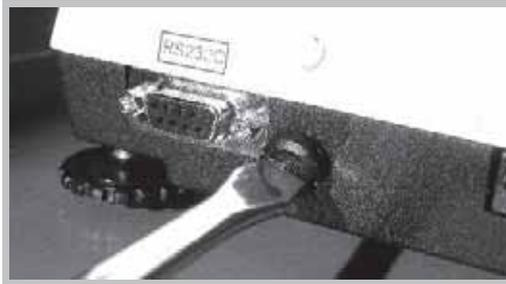
2. Once the screw has been removed and the calibration switch exposed, use a pen or another pointing device to toggle the calibration switch to the right (which is the ON position.)
