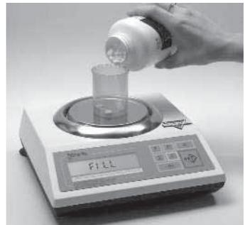
**Note:** If filling does not begin while the command "Fill" is displayed, after approximately 5 seconds the scale will display 0 pcs
