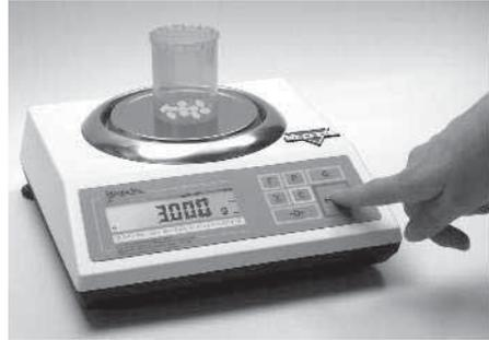
**Note:** Minimum individual piece weight allowed is 30mg (3e). With a sample size of 10 pieces, the sample weight must be equal to or greater than 300mg (30e). Attempting to set a sample size of 10 pieces with a total sample weight which is lower than 300mg (30e) will result in a Sample Low error (SAPL-LO)
