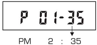
8. Upon pressing the T key, the hour digit will begin to change. In order to adjust the hour digit, press the T key while the correct hour digit is displayed. Per our example, if the time is 2:35 p.m., wait until the digit changes to a 2, and press the T key while 2 is displayed.
