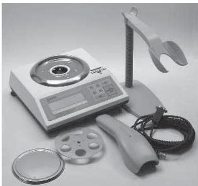
2. After removing the pan base and the pan from their packaging, carefully install the pan base onto the scale by placing it on the pan support located in the middle of the scale. Once the pan base has been installed, carefully place the pan on the base as shown below.
