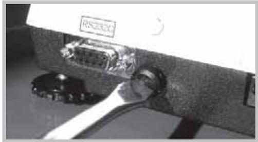
2. Once the wire seal screw has been removed and the calibration switch exposed, gently insert the flush sealing screw provided with the scale in the place of the wire seal screw.
