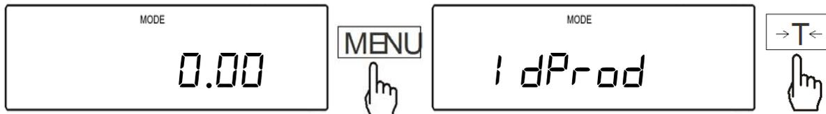
2. A dashed line will be displayed indicating to manually enter ID number. To manually enter the ID number, use the following keys: the C key to increment a digit, the T key to accept and go to the next digit, the
