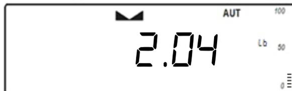
3. Once the stabilization indicator appears on the display, the container is ready to be tared. To tare the container, press the “T” button. The display will show a dotted line which indicates the scale has begun the taring process.
