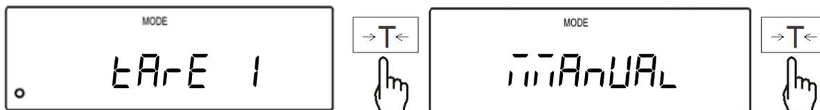
3. A dashed line will be displayed indicating to manually enter the Tare value. To manually enter tare value, use the following keys: the C key to increment a digit, the T key to accept and go to the next digit, the
