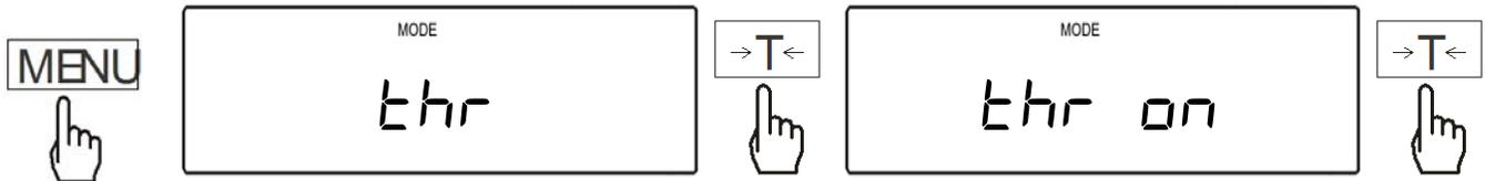
2. The scale will begin to display threshold limits. To set the Lower Limit waits for “Set-1” to display and press the T key. To set the Upper Limit waits for “Set-2” to display and press the T key. To set the minimum weight value that should be used in check weighing select “Set-3”.
