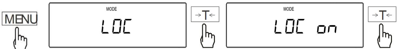
3. Place the animal or the moving object on the pan. Weight integration will begin automatically. If “LOC Prn” was selected press the data transfer key
