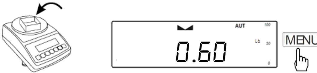
2. When the option “Tare” is displayed press the T key, and then select the option “Tar Set ” by pressing the T key once again.
