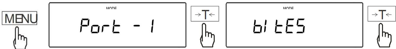
2. The scale will display available Bits settings: “7-bit”, ”8-bit”. To make a selection press the T key when the desired setting is displayed.
