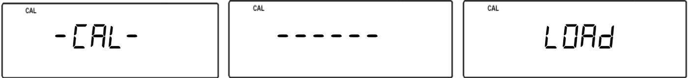
5. When the message “LOAD” is displayed, place the calibration weight on the scale’s hanging pan. Calibration will begin automatically and “WAIT” will be displayed indicating that calibration is in progress.
