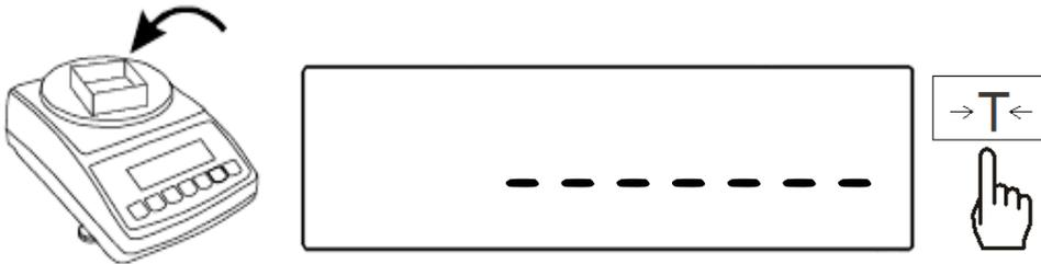
2. Press the Menu key, when the option “LOC” is displayed press the T key, and then select the option “LOC On” or “LOC Prn” by press the T key once again.
