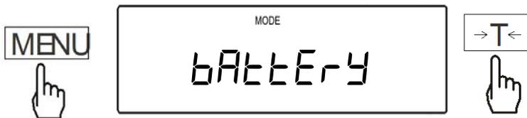
2. The scale will display options “BAT OFF”, “BAT ON”, “BAT VOL”. To disable battery charging press the T key “BAT OFF” is displayed, to enable battery charging press the T key when “BAT ON” is displayed.
