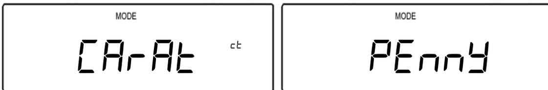
4. When the desired unit is displayed, press the T key to make the selection.
