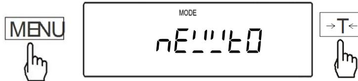
2. The scale will display options “ON” and” Off”. To enable Newton force measuring press the T key when “New On” displayed, to disable Newton force measuring press the T key when “New Off” is displayed.
