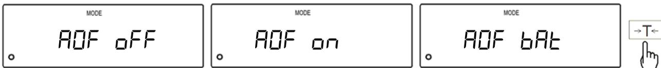
6. To make a selection press the T key when desired back light setting is displayed.
