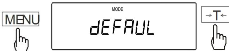
2. The scale will display options "Yes" and "No". To restore the scale's factory setting press the T key when "Yes" is displayed. To cancel press the T key when "No" is displayed.
