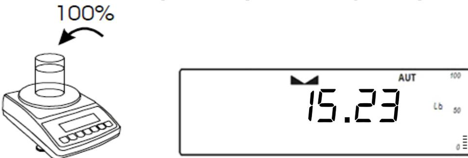
3. The weight of the sample will be displayed as it is placed on the pan. Once the weight of the sample stabilizes and the stability indicator appears on the display, press the MENU key to enter the main menu.
