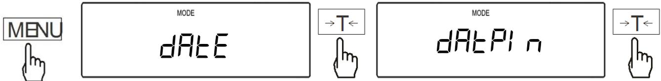
2. The scale will display a dashed line indicating to enter a desired PIN. To enter the PIN, use the following keys: the C key to increment a digit, the T key to accept and go to the next digit, the
