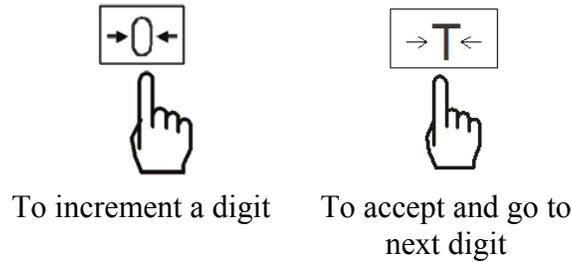
4. Once the time has been set the scale will display “PM” or “AM”. Press the T key when the desired setting is displayed.
