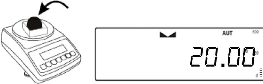
6. To obtain the gross weight (Tared container + unknown weight) press the B/G key.
