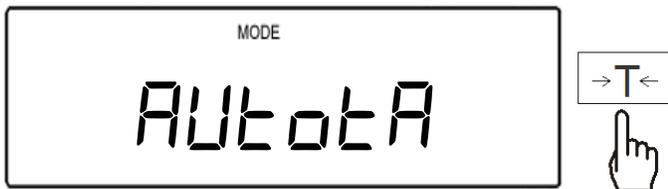
3. To enable Auto-zero press the T key when “Aut on” is displayed, to disable press the T key when “AutoFF” is displayed or select “out” to exit.
