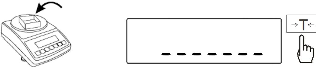
2. Press the MENU key, when the option “Total” is displayed press the T key, and then select the option “Tot o ” or “Tot –“ by press the T key once again.
