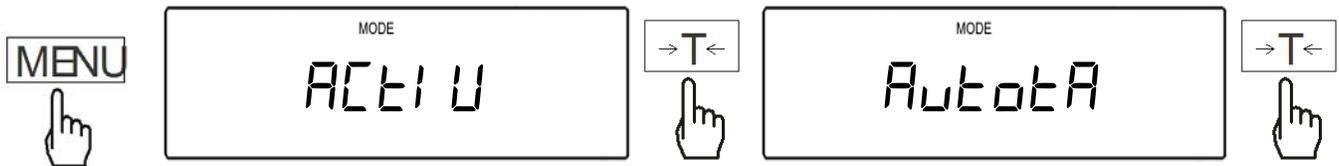
2. The scale will display options "ON" and "Off". To disable a function from appearing in the Main Menu press the T key when "Off" is displayed, to enable a function to have it appear in the Main Menu press the T key when "On" is displayed.
