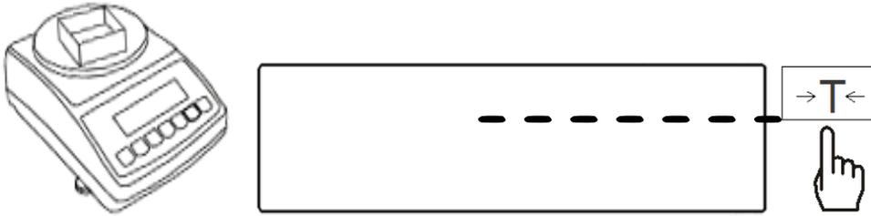
4. When finished taring, the balance will return to weighing and the NET indicator will be lit. The display will indicate 0.00g.
