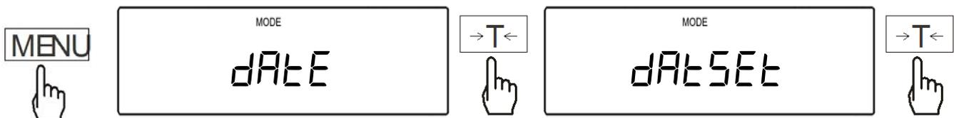
2. The current time will be displayed. To change or to set a new time press the T key
