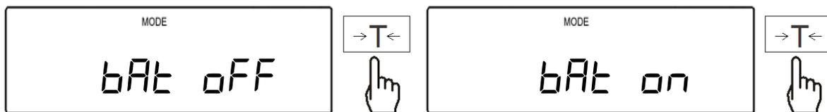
3. To check the batteries charging status press the T key when “BAT VOL” is displayed.
