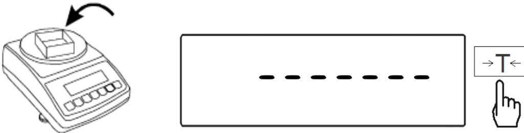
2. Place a sample in the container. The sample size must equal to one of the pre-set options: 5,10,20,50,100, 200,500, and press the MENU key
