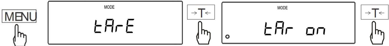
2. The scale will begin to Display tare locations. Locations marked with a dot in the upper left corner of the LED have a stored tare value assigned. To select a tare location press the T key when a desired location is displayed.
