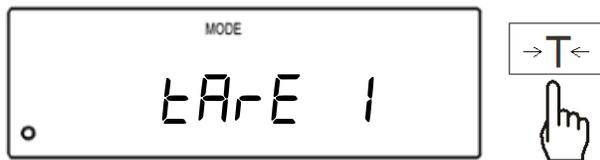
3. The scale will return to the weighing mode with the selected tare value in use.
