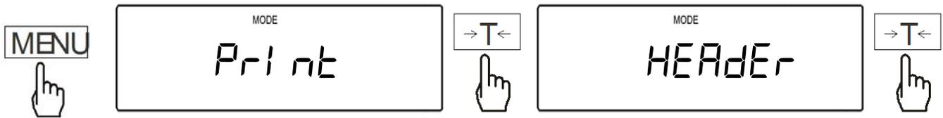
2. The scale will display options “ON” and” Off”. To enable the field press the T key when “On” displayed, to disable the field press the T key when “Off” is displayed.
