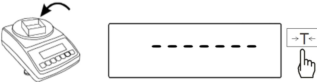
2. Once the scale has been tared, place the sample reference weight on the pan.
