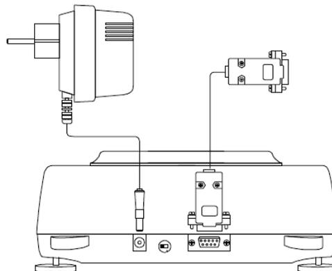
5. When the AC adapter is plugged into the wall outlet, the scale will turn “ON” automatically, initialize itself, and enter weighing mode.
