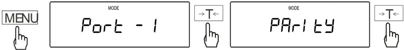
2. The scale will display available Parity settings: “none”, “odd”, “even”. To make a selection press the T key when the desired setting is displayed.
