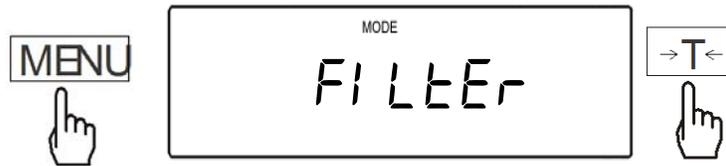
2. The scale will display options “Off” and available filter sensitivity levels “Fil 10, Fil 20, Fil 30 and Fil 40”. To select and enable Filtering press the T key when a desired filter level is displayed.
