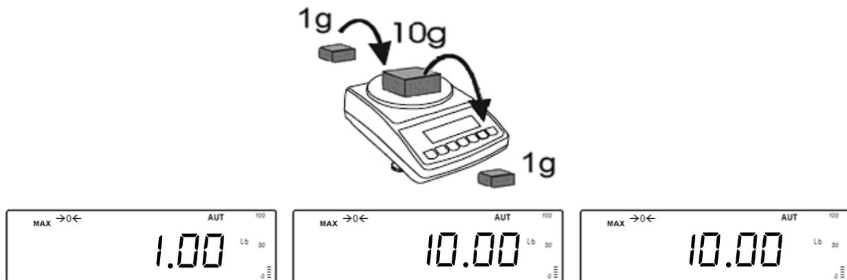
**Note:** Stability indicator and Auto-Zero is disabled during Min/Max weighing.
