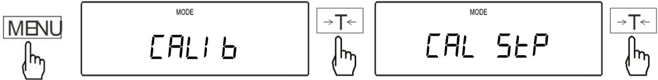
2. The scale will display a full a calibration mass equal to the scales capacity i.e.”30”, and an option to select a different calibration mass”other“. To calibrate the scale with a mass value equal to the scales capacity press the T key when the calibration mass value is displayed (proceed to step 4). To calibrate the scale with a mass lower than the scale’s maximum capacity, press the T when “other” is displayed (proceed to step 3).
