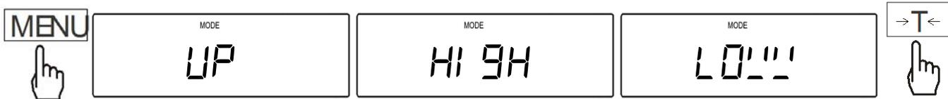
2. The scale will return to weighing and it will begin to hold on the display the highest or the lowest weight. When seeking the highest weight in a series make sure to remove the previous weight from the pan before adding the new weight. When seeking the lowest value weight be sure to add the new weight before removing the previous weight.
