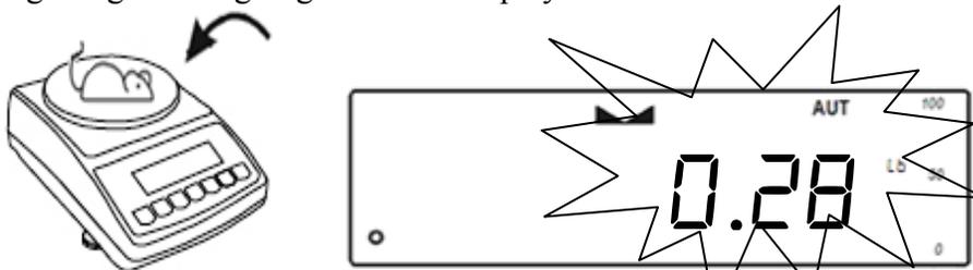
4. Final result will be automatically sent to a printer or a PC via the RS232 port. During data transmission the word print will be displayed. The final result remains displayed for 30 seconds. To perform the next weighing remove the animal, wait for the scale to display 0 and place the next animal on the pan.
