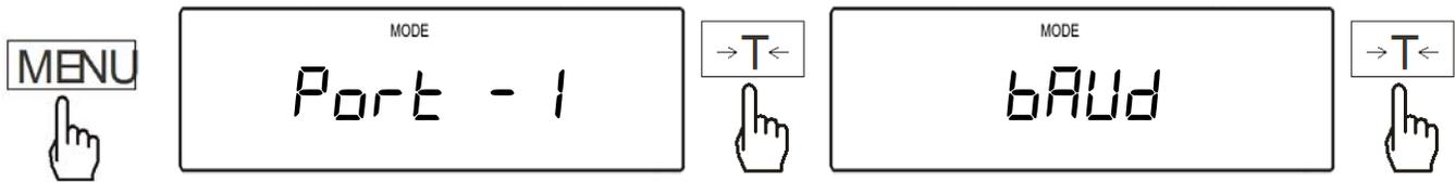
2. The scale will begin to display available baud rates: “4800”, “9600”, “19200”, “38400”, and “57600”. To make a selection, press the T key when the desired setting is displayed.
