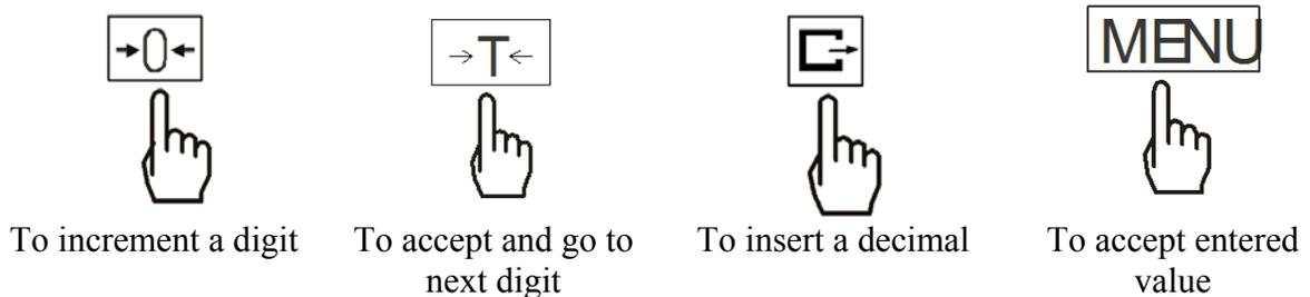
4. The scale will display the message “Press Menu”. When you are ready to Tare the scale Press the MENU key.
