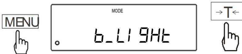
2. The scale will display available back light settings: “B\_L On”, B\_L Off, “B\_L ECO” and “B\_L BAT”.
