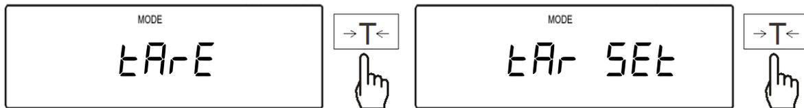
3. The scale will begin to Display tare locations. Locations marked with a dot in the upper left corner of the LED have a stored tare value assigned. To select a tare location or overwrite a current location press the T key when a desired location is displayed, and then select the option “Pan ” by press the T key once again.
