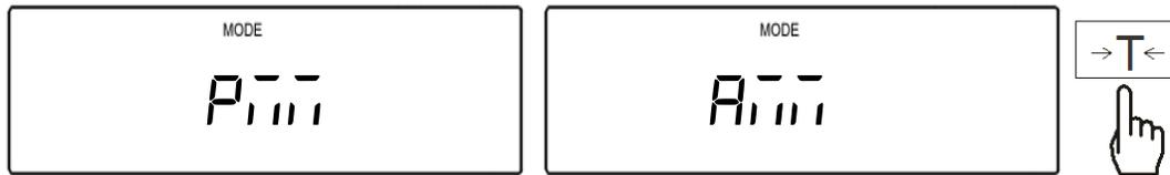
5. Once the Time has been set, the scale will display the current date. To change or to set a new date press the T key
