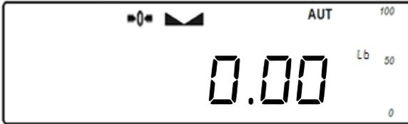
2. When weighing, always place the mass in the middle of the pan. The weighed result may be taken when the stabilization indicator appears on the display.
