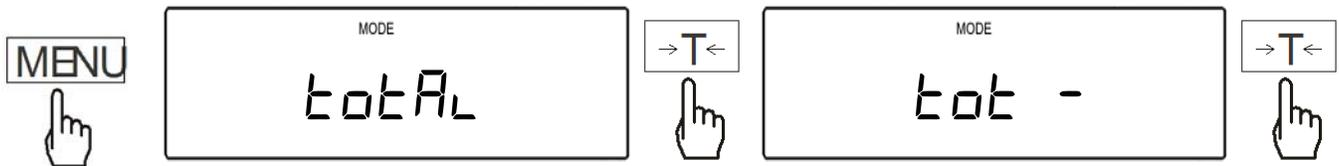
3. The display will read 0 indicating that you may place the first object into the container. Once the Weight of the object stabilized press the data transfer key
