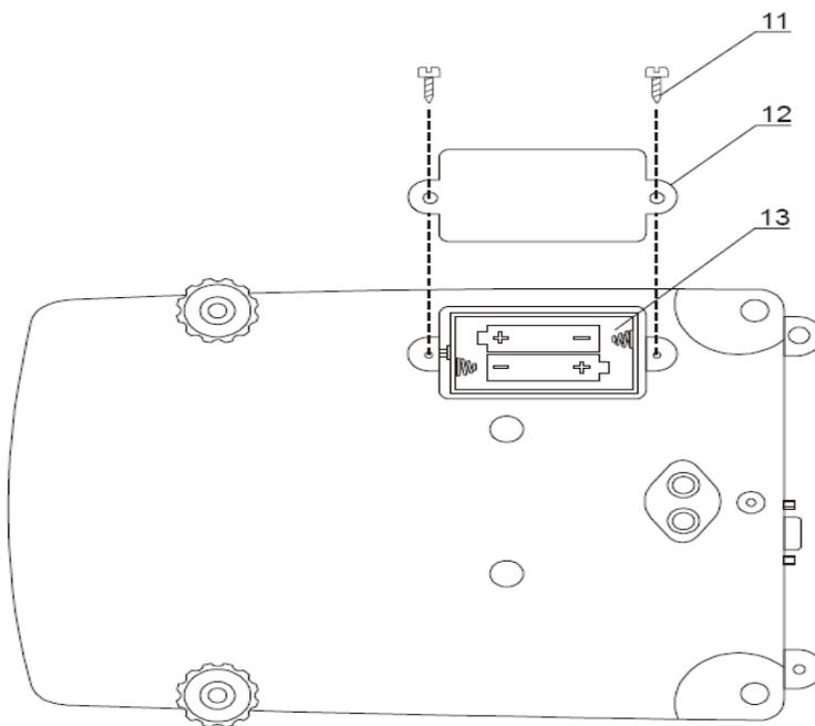
1. Remove the scale’s pan, pan base, as well as the draft ring (BTA200 Models) and carefully place the scale up-side down.
