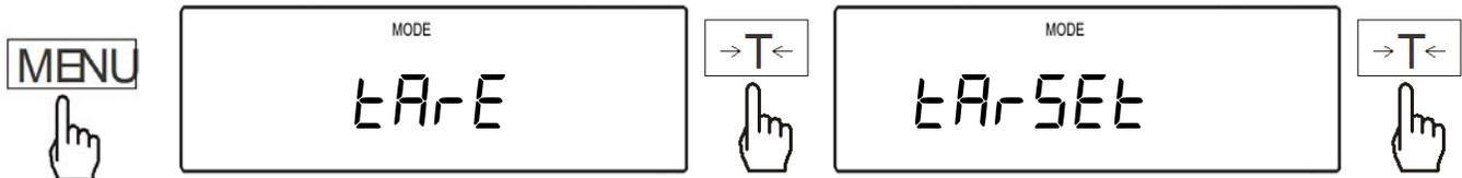
2. The scale will begin to Display tare locations. Locations marked with a dot in the upper left corner of the LED have a stored tare value assigned. To select a tare location or overwrite a current location press the T key when a desired location is displayed, and then select the option “Manual ” by press the T key once again.
